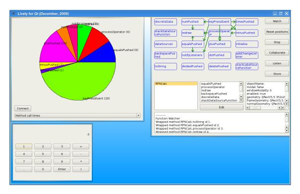
Figure A.5: Introspector examining RPN calculator instance while providing Charter method call statistics.
