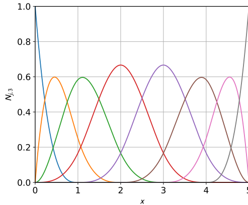
Figure 19: One dimensional cubic ( k = 3 ) B-spline basis functions on an open uniform knot \mathcal{E} = \{0, 0, 0, 0, 1, 2, 3, 4, 5, 5, 5, 5\} . There are 8 nodes (control points in CAD terminology) and 5 elements (or knot spans in CAD). As can be seen from the figure, at any point there are 4 ( = k + 1 ) non-zero basis functions. Therefore each element has 4 nodes. The first element's connectivity is [1, 2, 3, 4] i.e. particles locate in this element contribute to nodes 1, 2, 3 and 4. The second element's connectivity is [2, 3, 4, 5] and so on [Hughes et al., 2005].
